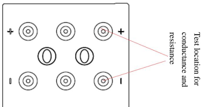
**Figure 3-3 Test location for conductance and resistance**
