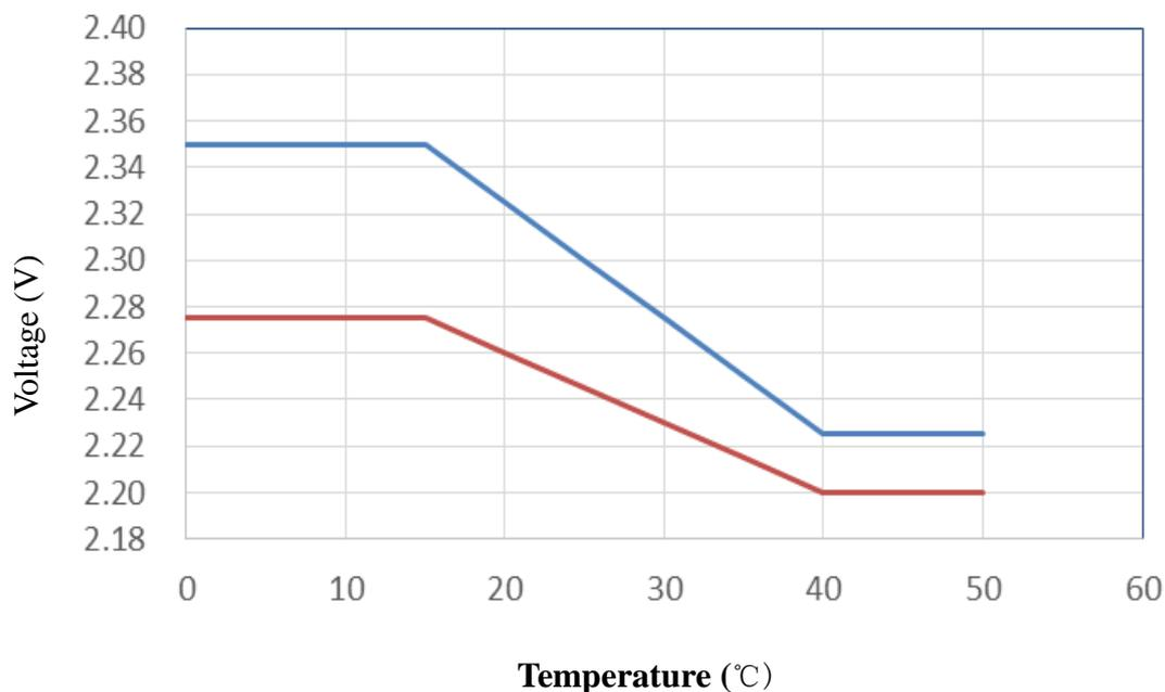
**Fig. 3 - 2 The Voltage Setting Curve Vs. Ambient Temperature**
