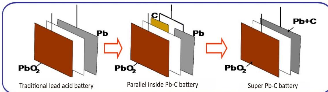
**Fig.1-2 Lead carbon battery working principle sketch map**
